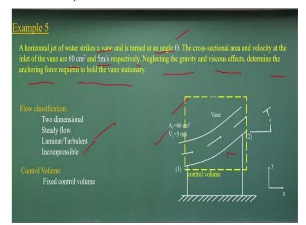
Now let us come to the example fifth which is again a simple problem where a horizontal jet of water strikes a vane, this is the vane, okay? Is turned the angle to theta degree. Cross-sectional area and velocity at the inlet of the vane is 60 centimeters, 5 meter per second respectively neglecting the gravity and viscous effect, okay?
