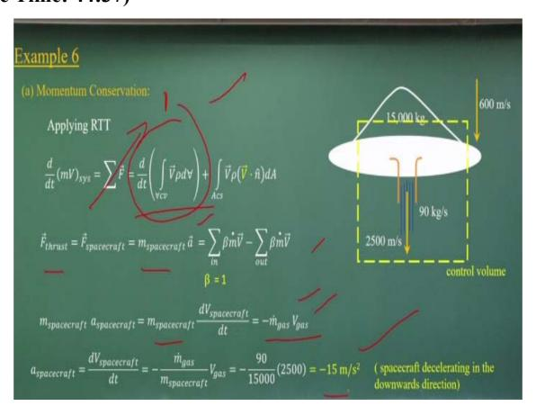
And let us apply the Reynolds transport theorems, okay. In this case, as we have considered earlier, okay. So there is this force component is zero. Only the change of the rate of the momentum flux within the control volume that what will force thrust,
