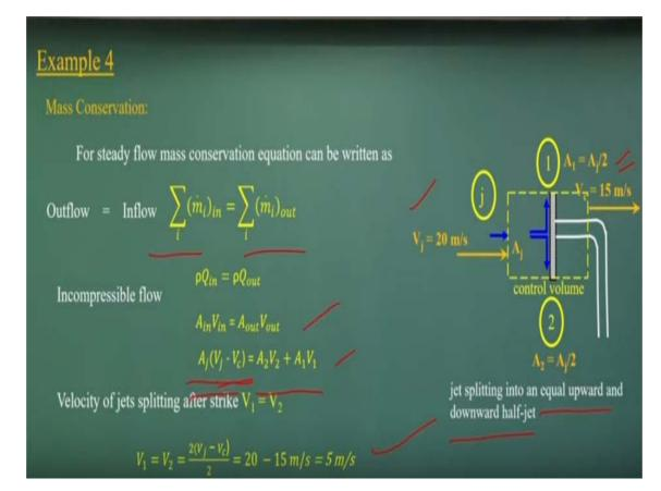
And if this is the V 1 to this cross section V z is water is coming into that and it is splitting into two part is equally part. So this is velocity of jet, this is what the moving control volume is moving with 15 meter per second. Jet is splitting into equally upward half-jet, the half of what goes to upward direction, half of water goes to the downward direction. If is that let us first apply the mass conservation equations.
