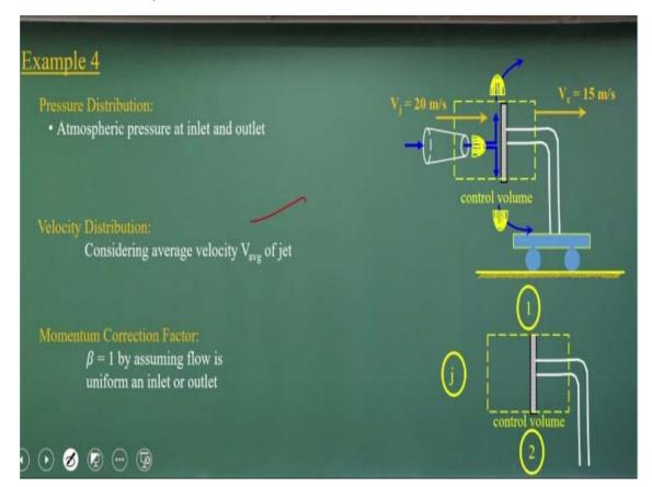
The pressure distributions in atmospheric pressure distributions will be the atmospheric pressure distribution the we will consider the average velocity conditions and the beta equal to the 1. Okay that the great simplifications we used to do it.
