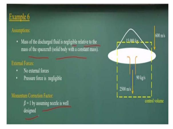
Now if I have a another assumption as you said, the mass of the discharged fluid is negligible, is relative to the mass of the aircraft. This will be the solid bodies moving with a constant mass, okay. No external forces. The pressure forces can be negligible. Beta is equal to the 1, assuming the nozzle is well designed, okay. So because a well designed nozzle have a close to the uniform velocity distribution. So beta will be 1.
