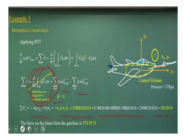
Now we have to find out what is the force acting in  $R_x$  and the  $R_y$  directions, we have the pressure component here. Applying this Reynolds transport theorems and the simplifying the tops. Here, this is the main concept what we have consider it that there is a change of the momentum flux within the control volume. But the right of the change of the momentum flux within a control volume, is not that significant order as compared with the momentum thrust what is coming from the fuel.
