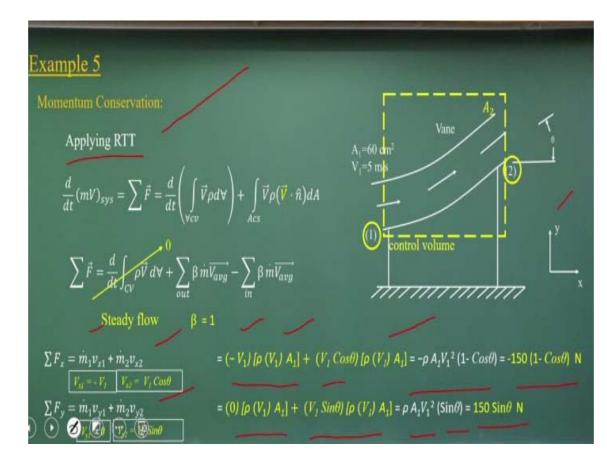
Now need to apply the momentum conservation equation, apply the Reynolds transport theorems to compute what will be the force. First again steady flow conditions which is standard assumptions we have been doing it for simplifying the problems for the problems here what we have considered it and  $\beta$  equal to 1.
