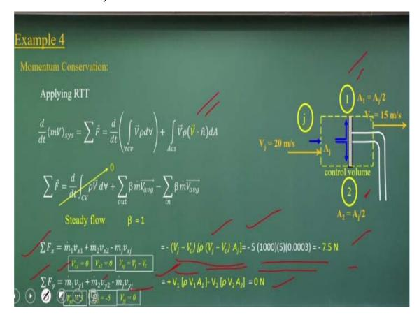
Now I am applying momentum conservation equation. We remember it I need to apply the relative velocity component here as the part the considerations here and beta equal to the 1 and I apply the relative velocity component. That what you can look it how the relative velocity components are used for the mass flux and the momentum flux component and that what is substitute to get it what is the force component. So the problem is similar nature.
