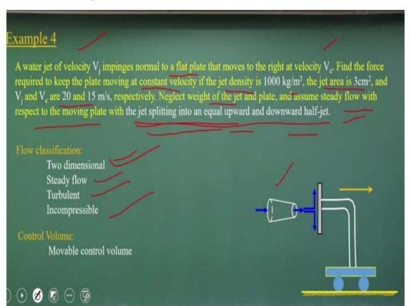
Like let we will have a water jet, the if you look it this is the water jet, is impinging this normal to a flat plate and moves to the right to the velocity V c, okay this that means, this flat forms is moving with a velocity V c. Find the force required to keep the plate moving at the constant velocity if jet density is this, the water density is this. Jet area is given and V j the velocity of water jet and the V c the velocity of the frame is respectively 20 and 15 meter per second.
