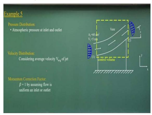
And the jet is there is atmospheric pressure and the velocity distribution again we can consider is a uniform. That is what not a conditions when you have the free jet in it going through the vane V but we can assume it the velocity distribution is uniform.
