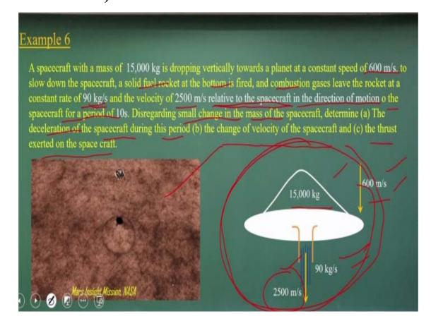
Let us see this, the figure what is showing is that when a spacecraft are landing on the surface, it decelerate it. It decelerate the terminal velocities and then it land on the earth or the any planets. So how do you do decelerate it? That is what we do it to decelerate that. It is the problems what you have consider it a spacecraft with a mass of 15000 kg dropping vertically towards a planet at a constant speed of 600 meter per second.
