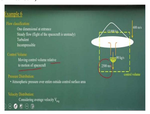
Now the problem is one dimensional because only one jet is there. We can use as a steady problems, turbulent, incompressible. This is a moving control volume, relative to motion of the space aircraft. Here we are talking about the relative velocities. We are not talking about the absolute velocity of jet and if it is that we consider the control volumes and try to find out what will be the force is acting because of this firing of the gases from this space aircraft.
