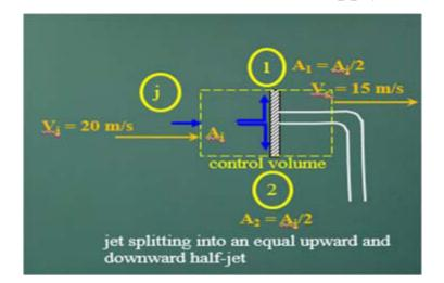
The mass influx is equal to mass outflux. If that is the conditions you have a these values, okay. Please remember it we consider here the relative velocity component along the and it has the  $V_1$ ,  $V_2$  velocity which is going out where the velocity components, we do not have any velocity components in the y direction. But is only moving in the x direction, that is the reason.
